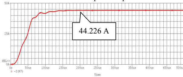
Fig. 4-2. Output current of the modulator with the current operation parameters
