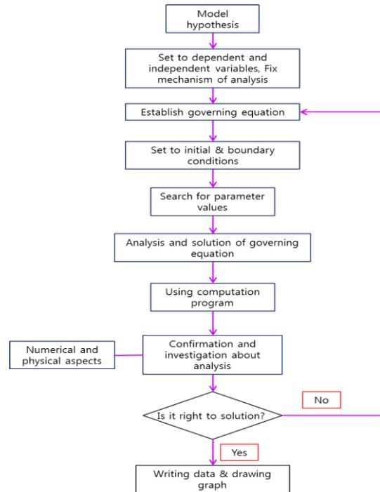
Fig. 2. Procedure of DU bed hydriding/dehydriding simulation to heat and mass transfer.
