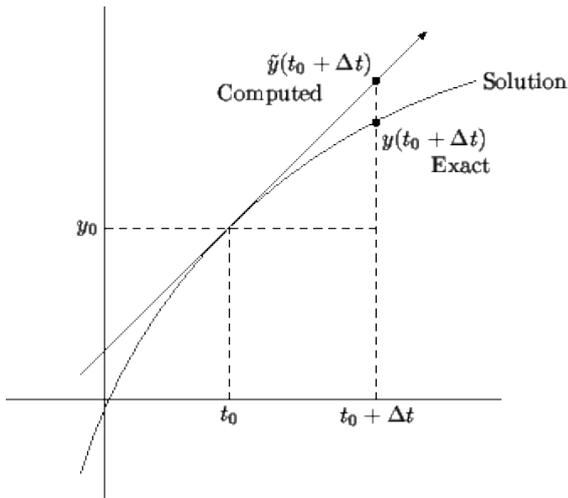
Fig. 1 Mathematical principle of Euler's method [8].
