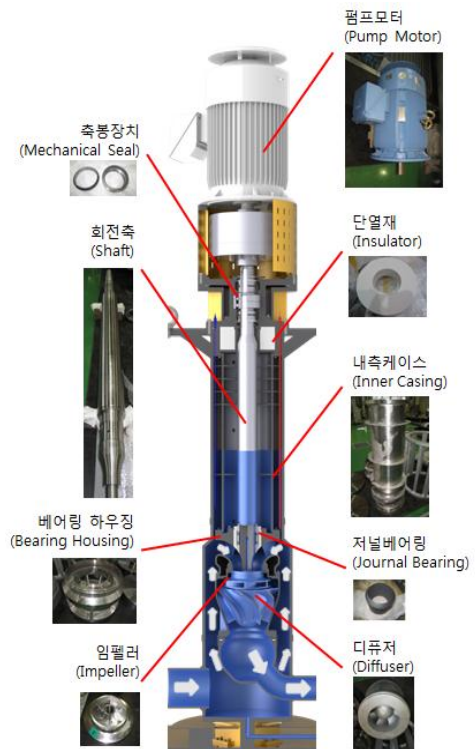
Fig. 2 Mechanical sodium pump in STELLA-1
