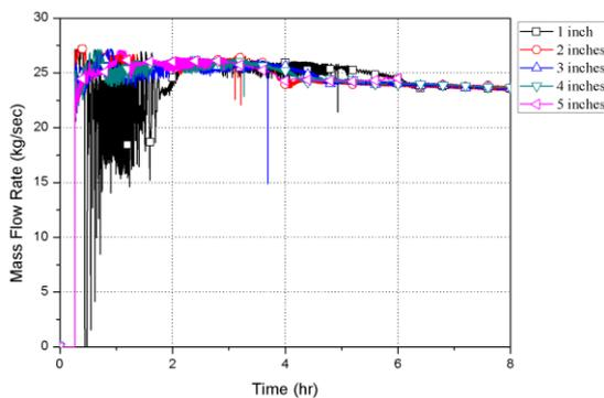
Fig. 3. Mass flow rate of SGGI-PDHR in IPSS
