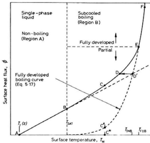
Figure 3. Wall temperature vs. Heat flux [13]
