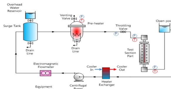
Figure 1. Schematic of experimental loop installed in KAIST [6]
