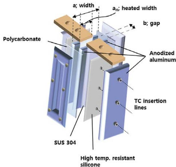
Figure 2. 3-D cut-view of test section [6]
