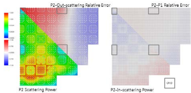
Fig. 8. Pin power distribution with P2 MOC and relative differences between each method and P2 for the VERA 5C case
