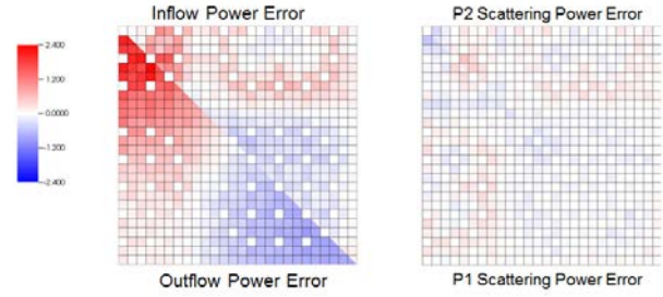
Fig. 4. Errors of pin power distribution of the 4C case with various transport corrections, P1 and P2 MOC method
