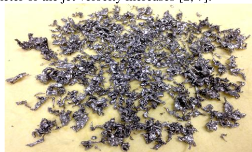
Fig. 6 Debris of molten wood's metal
