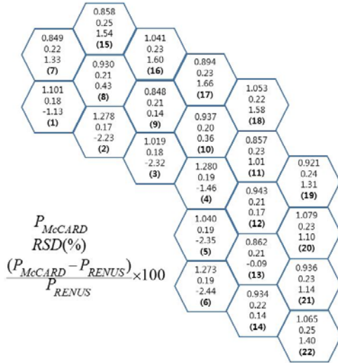
Fig 3. Comparison of radial relative power distribution of McCARD with RENU S results
