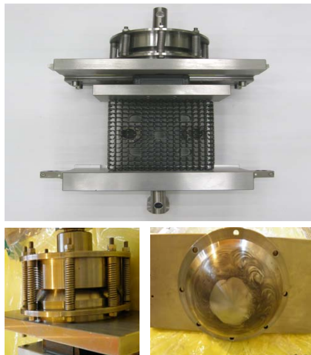
Fig. 3. The compression test device composed of lower and upper plates with a spherical bearing.
