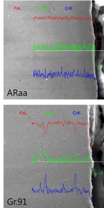
Fig. 5. Elemental distribution at the corroded surface.
