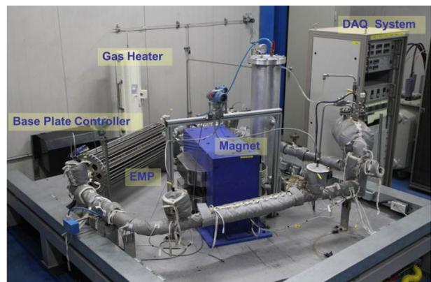
Fig. 1. A photo of the experimental loop.
