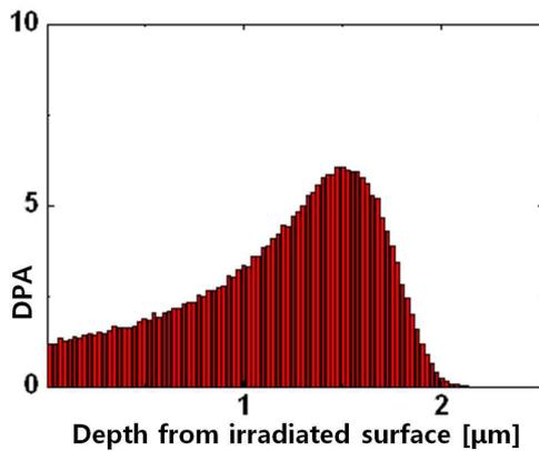
Fig. 1. Estimated depth of the damaged layer using Monte Carlo simulation code (SRIM 2012)
