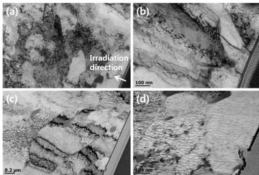
Fig. 2. Radiation-damaged area of the ARAA alloys were shown. The microstructure of the F/M-1, (a) 0-2.5  $\mu\text{m}$  deep from the surface, (b) typical morphology of damaged area. The similar microstructure of the F/M-2 were shown in (c) and (d), respectively. Lots of point and line defects were found, no specific voids were observed.
