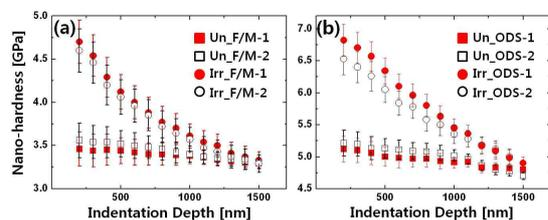
Fig. 4. Nano-hardness were measured on the surfaces of the un-irradiated and the irradiated specimens. Nano-hardness of (a) F/M steel, (b) ODS steel were measured by the differentiating indentation depth, respectively.
