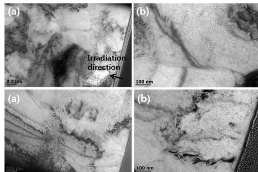
Fig. 3. Radiation damaged area of the ODS alloys were shown. The microstructure of the ODS-1, (a) 0-2.5  $\mu\text{m}$  deep from the surface, (b) typical morphology of damaged area. The similar microstructure of the ODS-2 were shown in (c) and (d), respectively. Small nano-sized circular shapes were observed, they were cavities.
