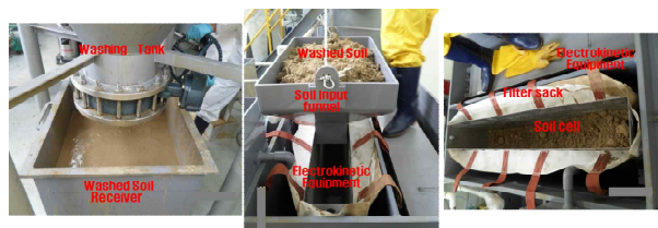
Fig. 1. A photograph of putting the washed soils into the electrokinetic decontamination equipment
