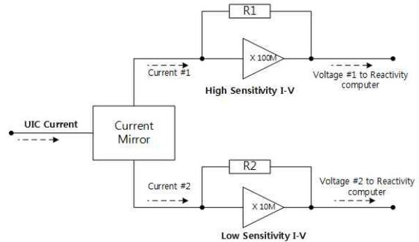
Fig. 1. Block Diagram of RCIC
