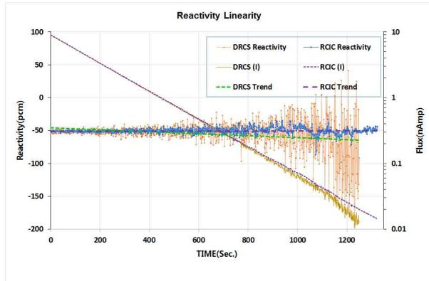
Fig. 2. Comparison of reactivity linearity for DRCS and RCIC
