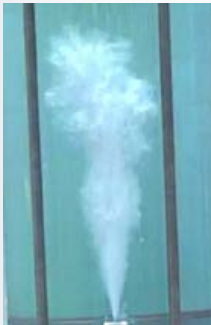
Fig. CO 2 -gas jet at 0.75MPa into water [D. Vivaldi et al., 2013]
