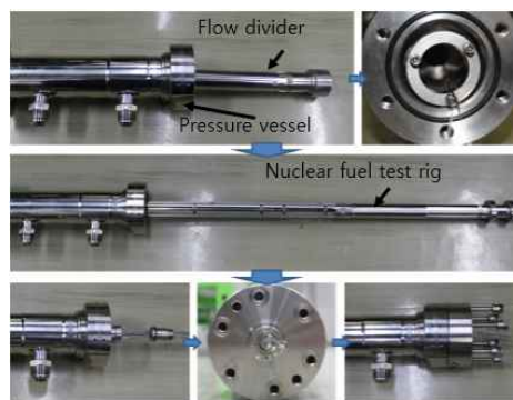
Fig. 4. Install of a nuclear fuel test rig in the pressure vessel.
