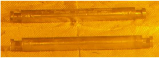
Fig. 2 2 Irradiated VHTR fuel rods after capsule dismantlement
