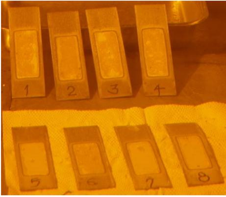
Fig. 1 8 Irradiated fuel plates after capsule dismantlement
