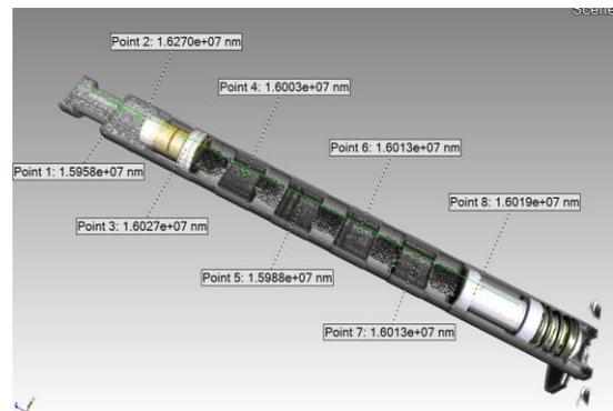
Fig. 7 Dimensional measurements of 2 VHTR rods by 3-D computer software
