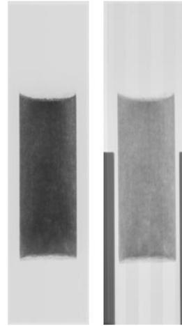
Fig. 5 Fuel meat shape before(left)/after(right) irradiation
