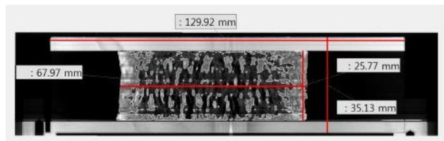
Fig. 6 Dimensional measurement of fuel plate by 3-D computer software
