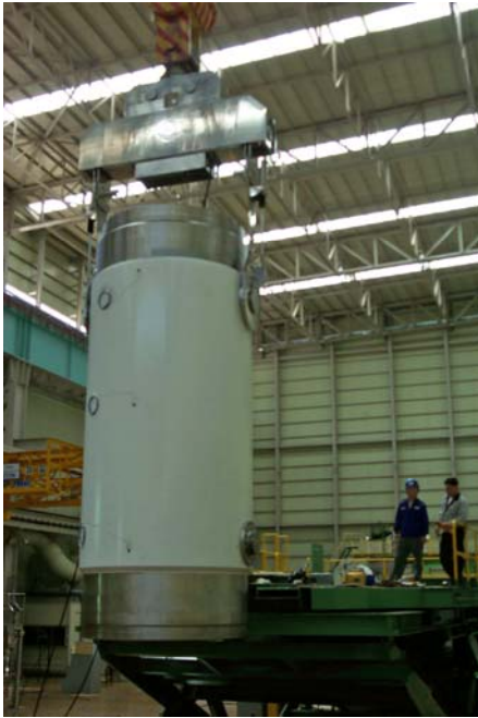
Fig. 8. CASTOR ® KN-12 for the wet transfer of spent fuel at Kori /S. Korea
