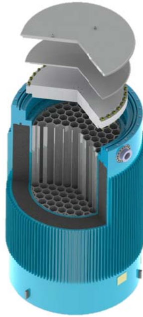
Fig. 9. Schematic diagram of a CONSTOR® cask for hexagonal FA
