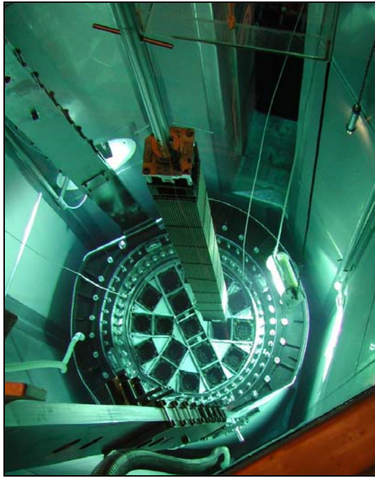
Fig. 1. Loading of a CASTOR ® V/19 for PWR-FA
