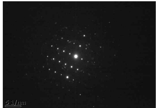
Fig. 2. SAED pattern of the simulated oxide layer.
