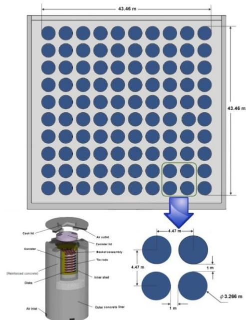
Fig.1. Schematic layout of ISF and concrete cask model.
