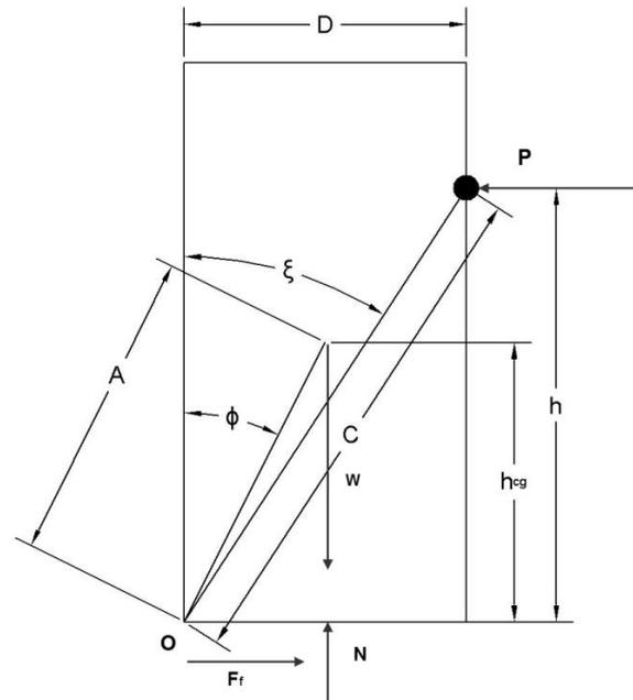
Fig.4. Free-body diagram (FBD) for storage cask.
