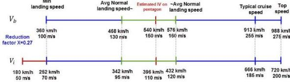
Fig.2. Description of measured velocity of B747 before and after collapse the storage-building wall.
