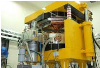
Fig. 1. Cyclotron KIRAMS-13 in Pusan National University
