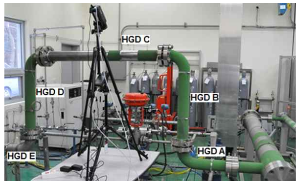
Fig. 4. HGD test section with IR cameras
