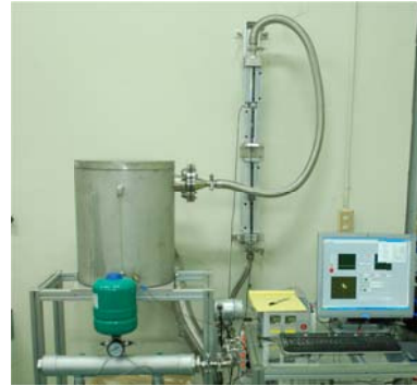
Fig. 1. Schematic view of FivWearRT used in this study. (Grid-to-rod fretting simulator for RT)
