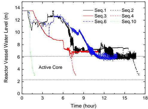
Fig. 3 Reactor vessel collapsed water level
