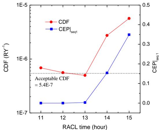
Fig. 6 Assessment Results According to the Reset of Offsite Power Restoration Time of Sequence 1
