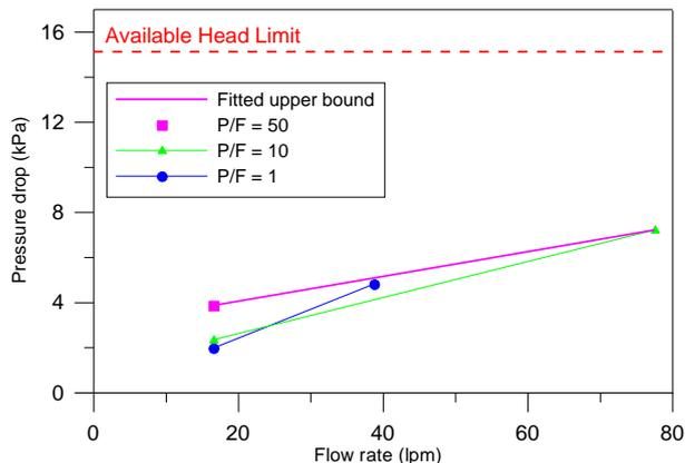
Fig. 5. Pressure drops vs. flow rates at different P/F ratios
