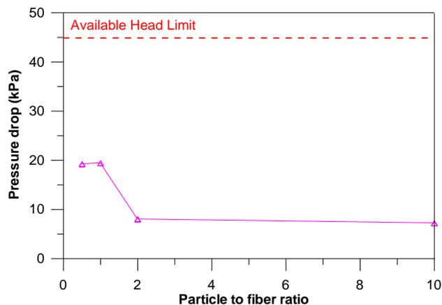
Fig. 4. Pressure drops vs. particle to fiber ratio under a hot-leg break condition
