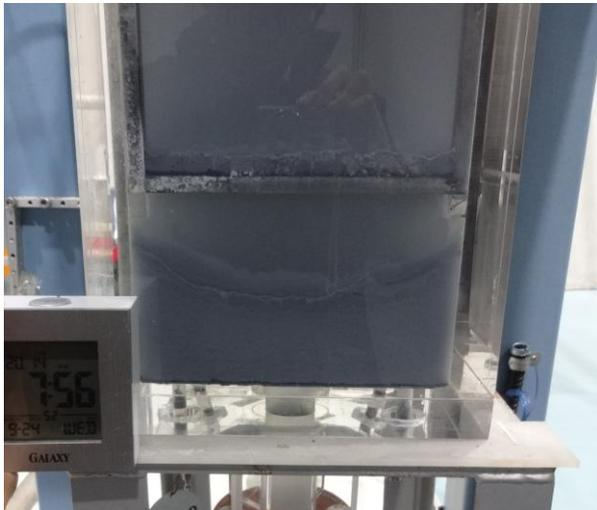
Fig. 1. Debris settling under the CL break tests
