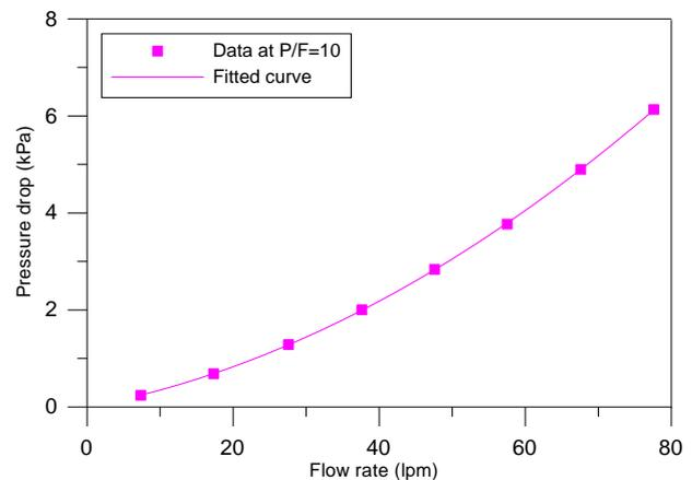
Fig. 2. Pressure drop dependence on the flow rate
