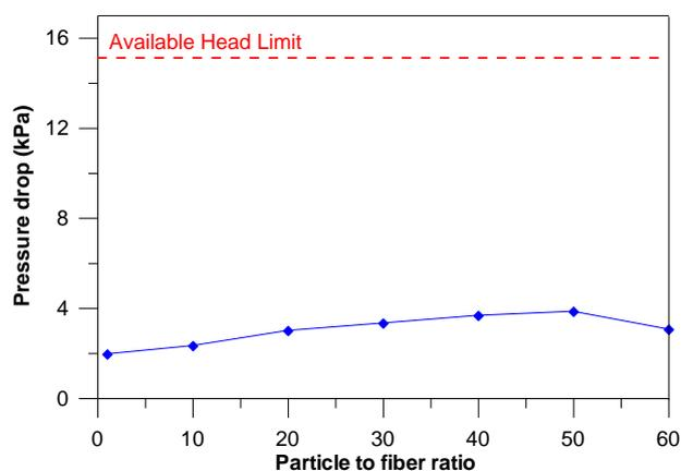
Fig. 3. Pressure drops vs. particle to fiber ratio under a cold-leg break condition
