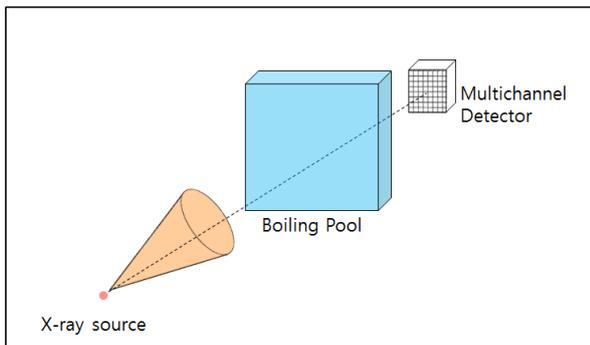
Fig. 1. Schematic Diagram of X-ray Based Flow Inspection System
