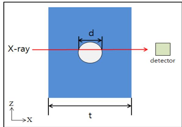
Fig. 2. Principle of the Bubble Size Detection
