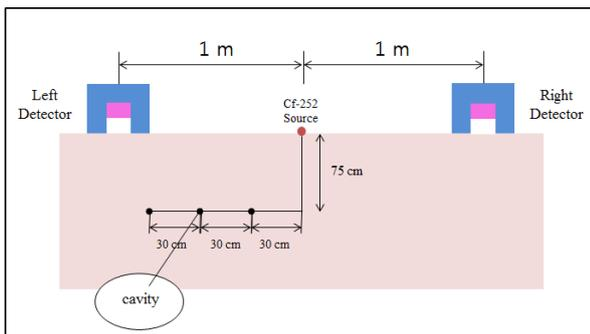
Fig. 1. Overview of the Detection System for the Feasibility Study
