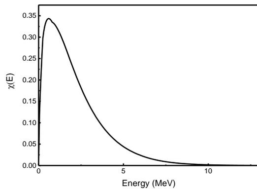
Fig. 2. Neutron Energy Spectrum of Cf-252 Source
