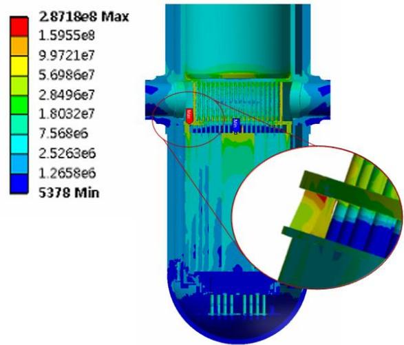
Fig. 5 Stress contour and maximum stress location
