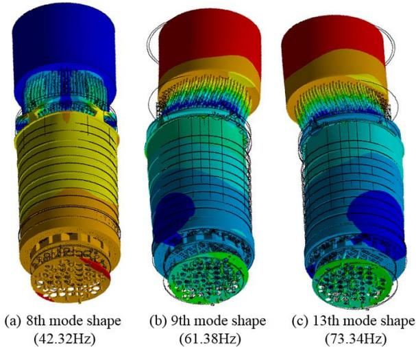
Fig. 3 Typical mode shapes of assembled RVIs
