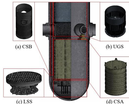
Fig. 2 Numerical model of assembled RVIs
