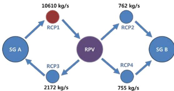
Figure 1 Flow distribution in RCS during on RCP operating
