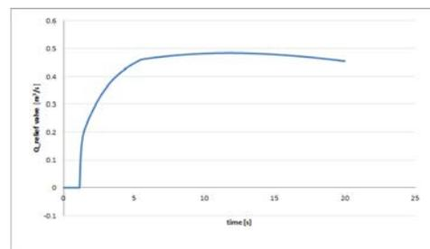
(a) Mass flow rate through LTOP relief valve
