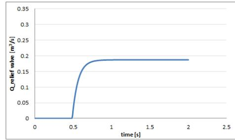
(a) Mass flow rate through LTOP relief valve
