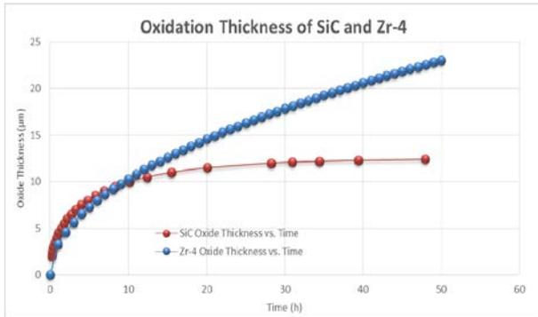
Fig.1: Comparison between Zr-4 and SiC Oxidation Behavior.
