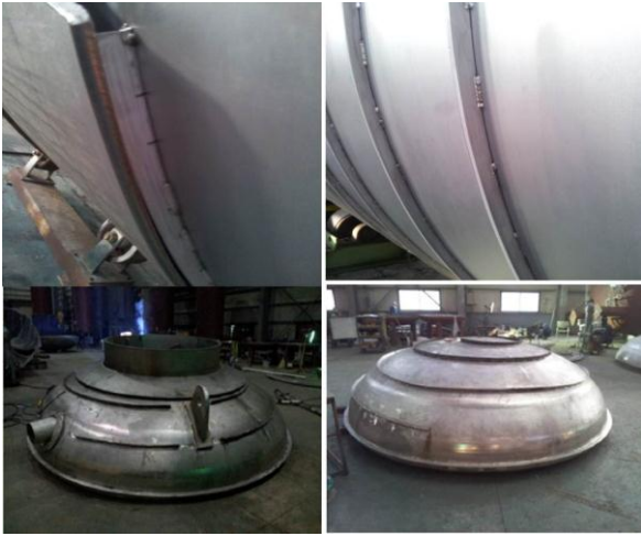
Fig. 2. Guiding panes welded on a pressure vessel [2].
