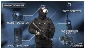
Among these, a SAT for a rifle offers convenience and economic efficiency when using electronic blank fire--which is simulated ammunition. Next, a player unit was manufactured in the form of a combat vest, which incorporates a detector set, effects simulator, and communication equipment. The detector sends real-time voice and location information within a radius of 2 km in combination with the DMR.
