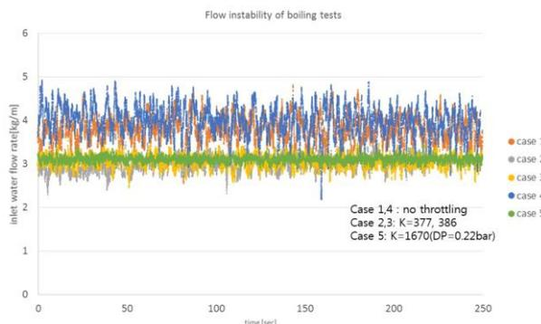
**Fig. 3.** Inlet mass flow rate instability of the boiling cases with different K-value
