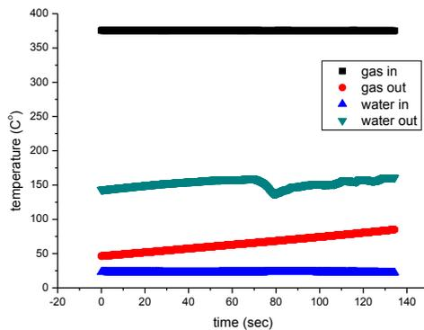
**Fig. 2** inlet and outlet temperature of helium and water during the superheated test
