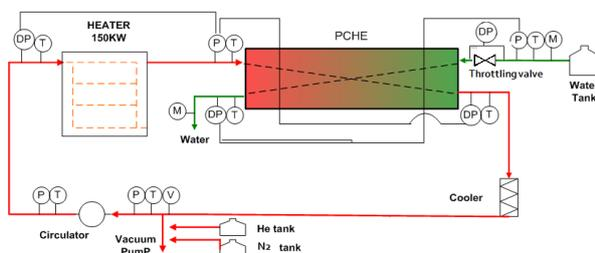
Fig. 1. Schematic diagram for PCHE test facility
