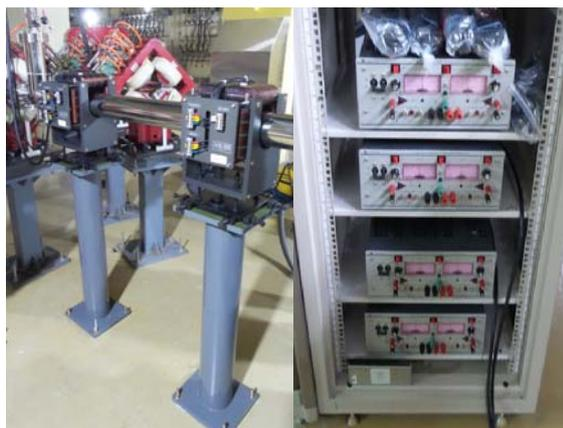
Fig. 5. Installation of steering magnet and power supply
