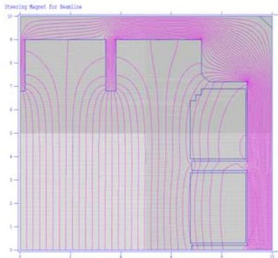
Fig. 1. 2D Poisson calculation for the steering magnet with 3-Ribs.
