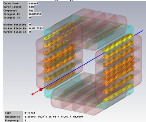
Fig. 2. Integration field of the steering magnet calculated by CST EM studio.
