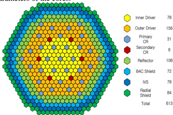
Fig. 1. Radial configuration of the cores
