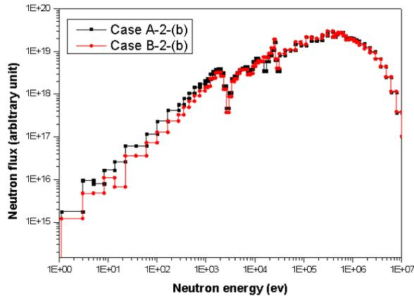
Fig. 4 Comparison of the neutron spectra for the cores having 12 moderator rods
