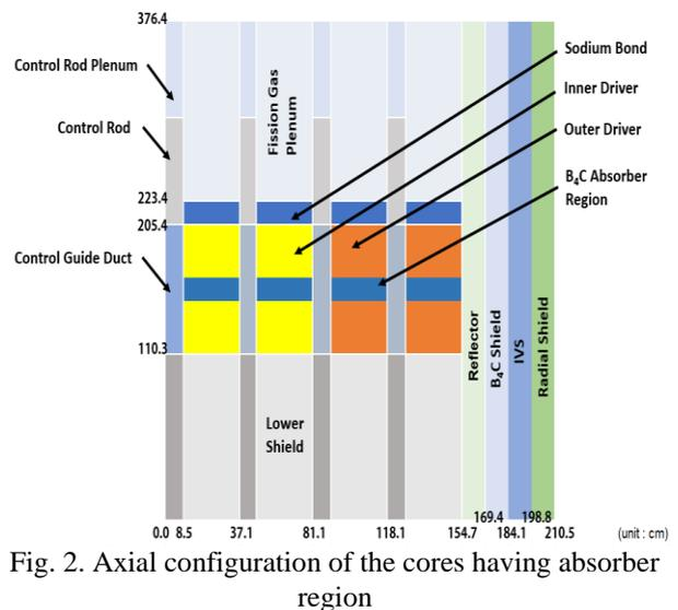
Fig. 2. Axial configuration of the cores having absorber region
