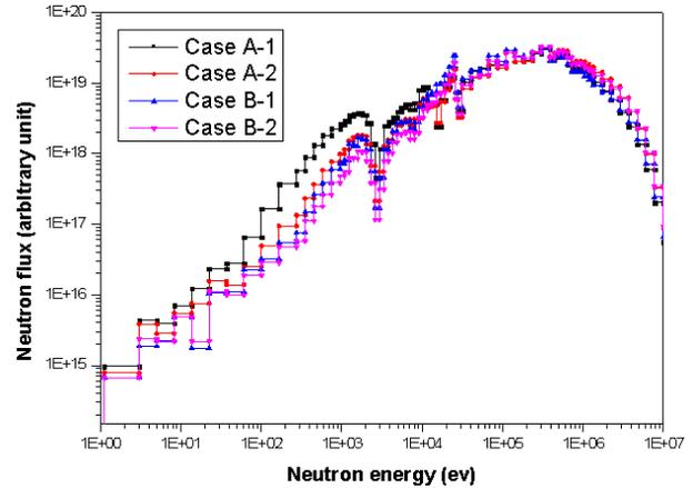
Fig. 3. Comparison of the core neutron spectra
