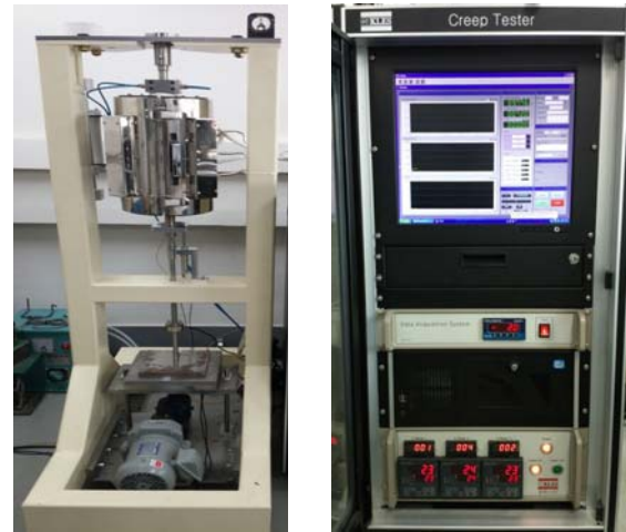
Fig. 2. Picture of the creep test apparatus and the data acquisition system.
