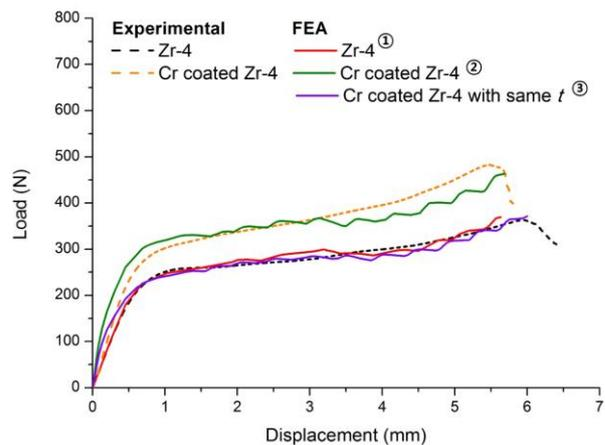
Fig. 2 Load-displacement results of RCT obtained from experiment and FEA simulation.
