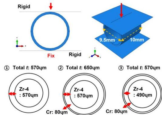
Fig. 1 Analysis model for ring compression test of coated fuel cladding and cladding model variation.
