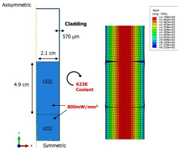
Fig. 3 Simply assumed PCMI simulation model and result of temperature distribution.
