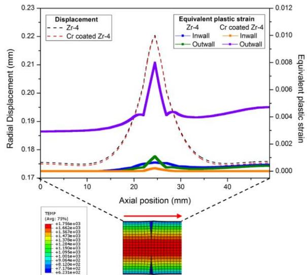
Fig. 4 Displacement and equivalent plastic strain of fuel cladding along the axial direction.
