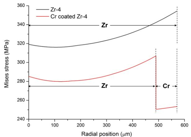
Fig. 5 Mises stress of fuel cladding along the radial direction.
