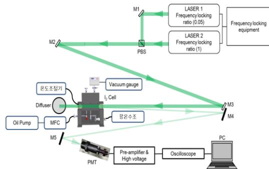
Fig. 2. Configured schematic for measurement of iodine gas with concentration using DIAL
