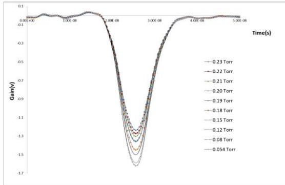
Fig. 3. PMT Signal for measurement of iodine gas with pressure using DIAL
