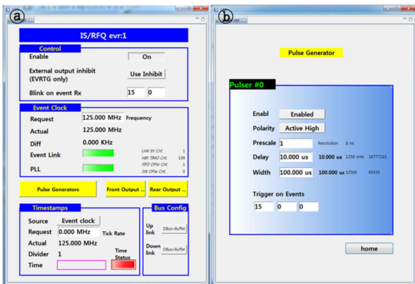
Fig. 5. OPI of event receiver: (a) and (b) panels for setting pulse output channel and pulse generator
