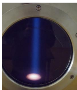
Fig. 3 Beam Shape of Duo-PiGatron Ion source for Vertical Type Ion Beam Facility (Nitrogen, 60keV 6mA)
