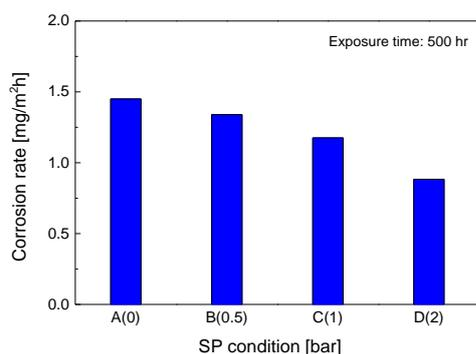
Fig. 2. Corrosion rate with SP air pressure.
