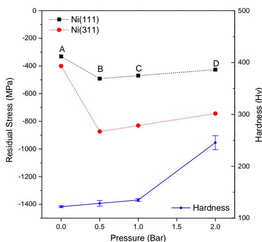
Fig. 1. Residual stress state and micro-hardness with SP air pressure
