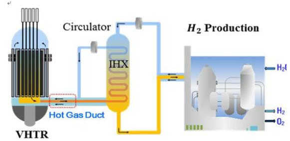
Fig. 1 Conceptual Layout of a Very High Temperature gas-cooled Reactor. (VHTR)
