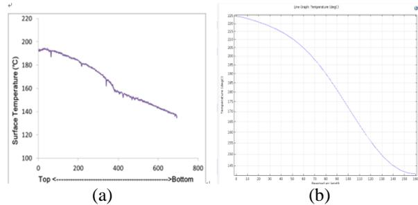
Fig. 5 Comparison of experiment and simulation results of surface temperature profiles at horizontal HGD.
