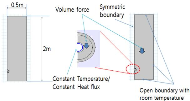
Fig. 3 Boundary conditions and geometrical model of a HGD in COMSOL 5.
