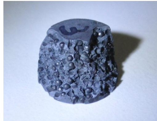
Fig. 3. Fracture surface of SiC matrix composite with 40 vol.% TRISO particles
