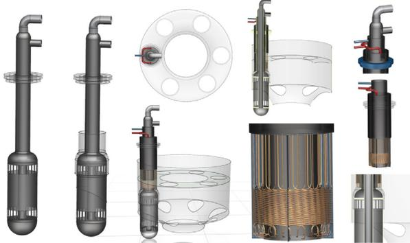
**Fig.2** Configuration of the CHX unit with 3D modeling
