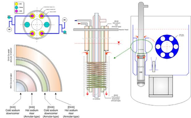
**Fig.1** Configuration of the CHX unit
