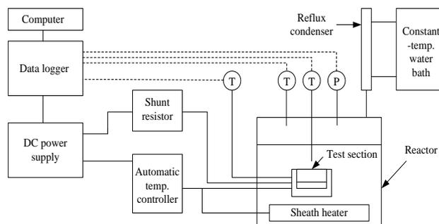
Fig. 2. Schematic diagram of CHF experimental apparatus.
