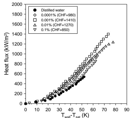
Fig. 4. CHF of oxidized graphene M-5 nanofluids.
