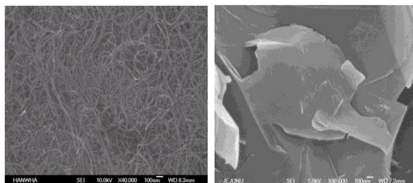
Fig. 1. SEM micrographs of MWCNTs and graphene.
