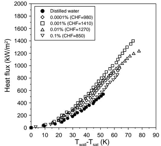
Fig. 3. CHF of oxidized MWCNT CM-100 nanofluids.
