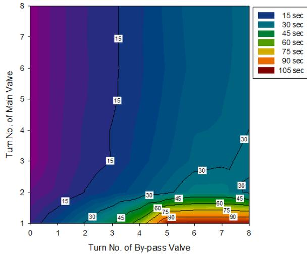
Fig. 3 Contour for withdrawal time at parametric performance test.
