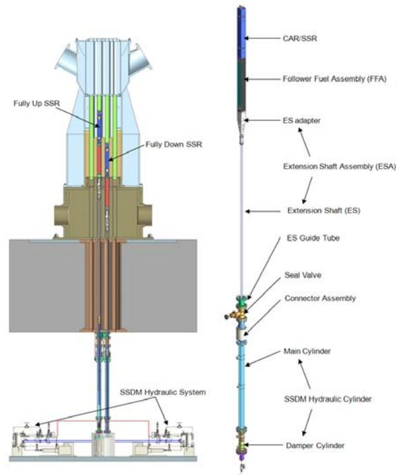
Fig. 1 Configuration of SSDMs.
