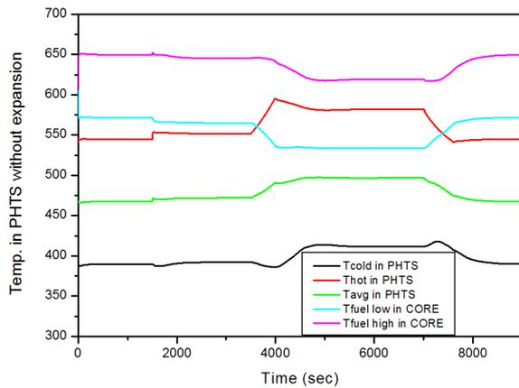
Fig. 5 Temperature of PHTS without expansion effect
