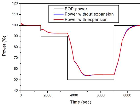
Fig. 1 Reactor Power according to BOP power.
