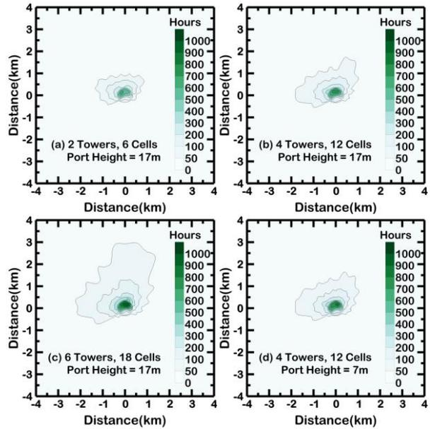
Fig. 2. Annual plume shadowing frequency for different cell numbers and port heights
