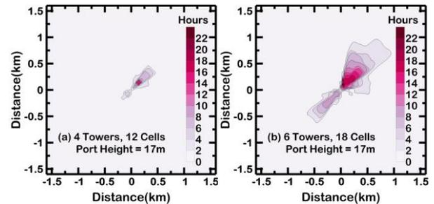
Fig. 3. Annual plume-induced fogging of APR1400DC LMDCT.
