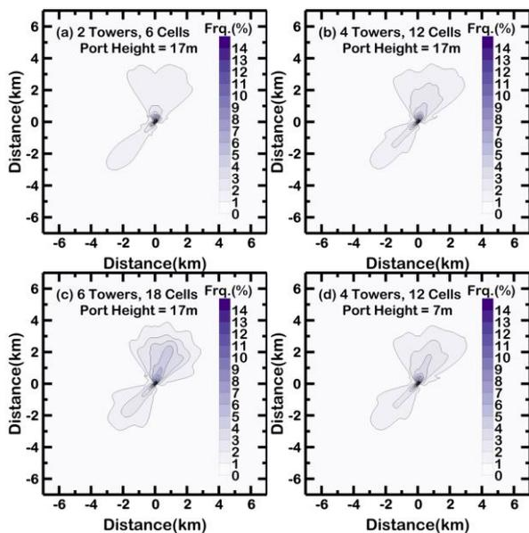
Fig. 1. Annual plume length frequency for different cell numbers and port heights
