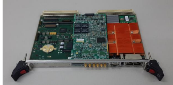
Fig. 1. IVME7210 baseboard and Pentek7156 FPGA PMC extended board.
