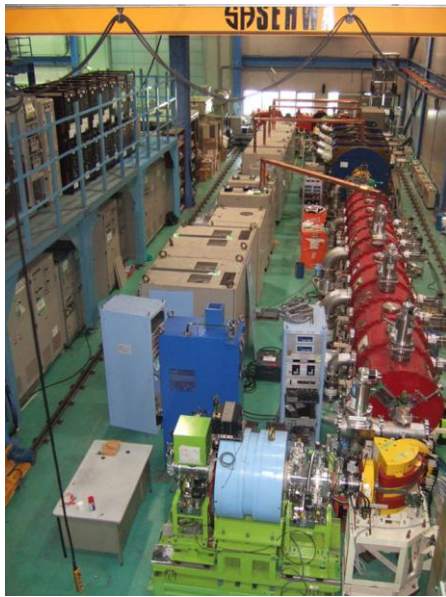
Fig. 2. Layout of the assembled main beam line of DIAC.
