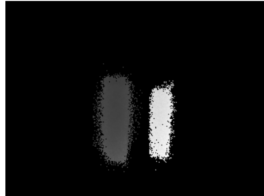
Fig. 5. Acquired range Image with an object discriminator from low-visibility fog environments.
